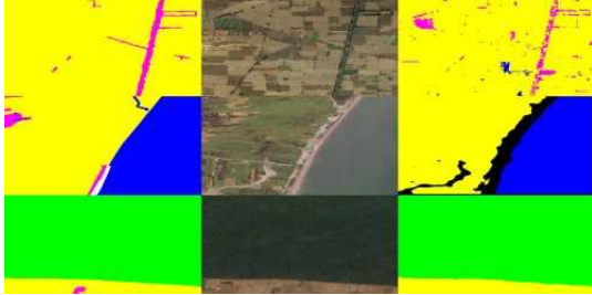
Figure 10: Remote Sensing Image Classification. Left: the result from baseline approach provided by [11]. Middle: the corresponding original image. Right: our classification result.
