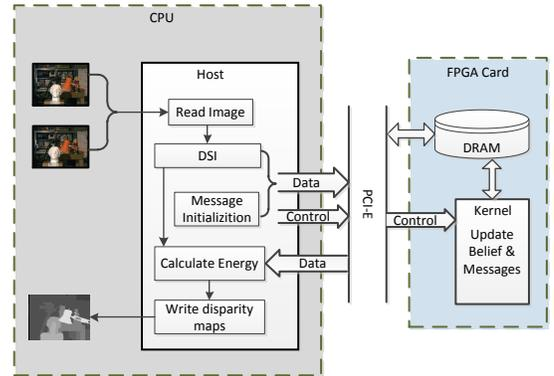
Fig. 2. Overview of the hybrid CPU/FPGA system
