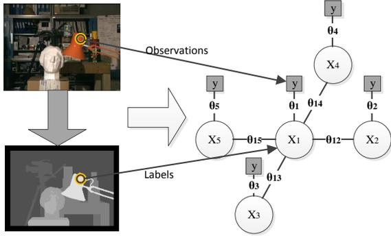
Fig. 1. Mapping a stereo matching problem to a 4-connected MRF
